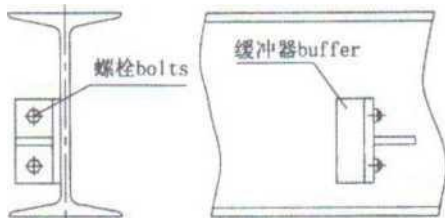
图 5 小车端部止档 Backstop at end of track of trolley
